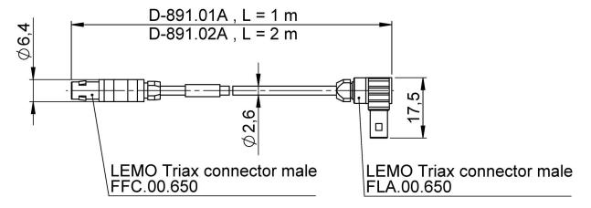
Usually the static bending radius is about 5-6x the diameter.
