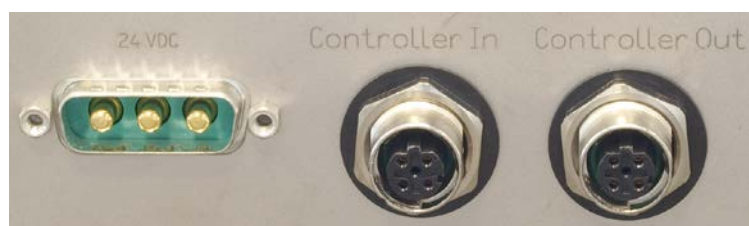
Figure 2: Connections at hexapod base plate
