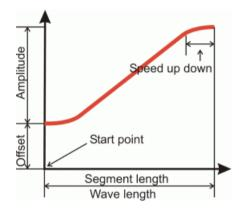
Note for the Sin\_P, RAMP and LIN wave types: If the <SegLength> value is larger than the <WaveLength> value, the missing points in the segment are filled with the endpoint value of the curve.
