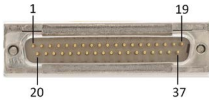
Figure 20: Sub-D 37 (m) piezo and sensor connection
