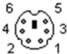
Figure 21: Front view of Mini-DIN socket
