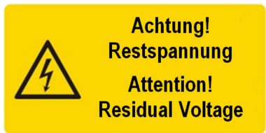
Figure 3: "Residual Voltage" warning sign on the connector of the U-651 Indicates risk of electric shock (p. 5)
