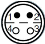
Figure 14: Sensor connection: LEMO connector FFA.05.304.CLAC32Y, contact side
