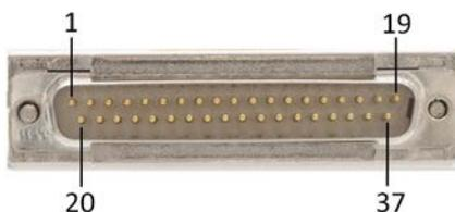
Figure 15: Voltage and sensor connection, sub-D 37 (m)
