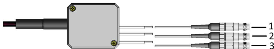
Figure 2: LEMO connections of the models without sensor
