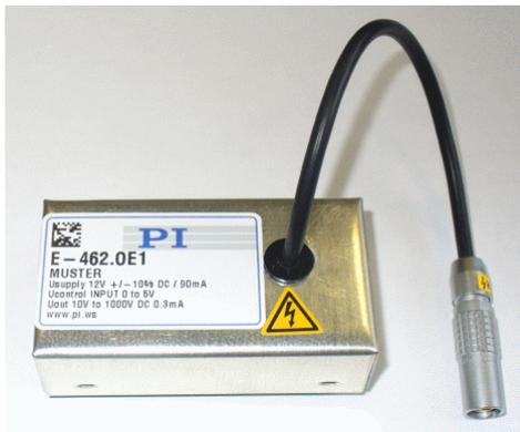
Figure 1: E-462.OE1 OEM module has HV cable on top and pins on the bottom (not shown) for PCB mounting
