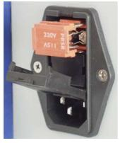
Figure 3: Position of the line fuses and fuse carrier, only one of two fuses visible
