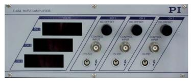
Figure 2: E-464 front panel with operating elements
