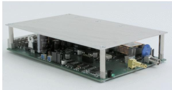
*Fig. 2: E-617.00F high-power piezo amplifier OEM module*
