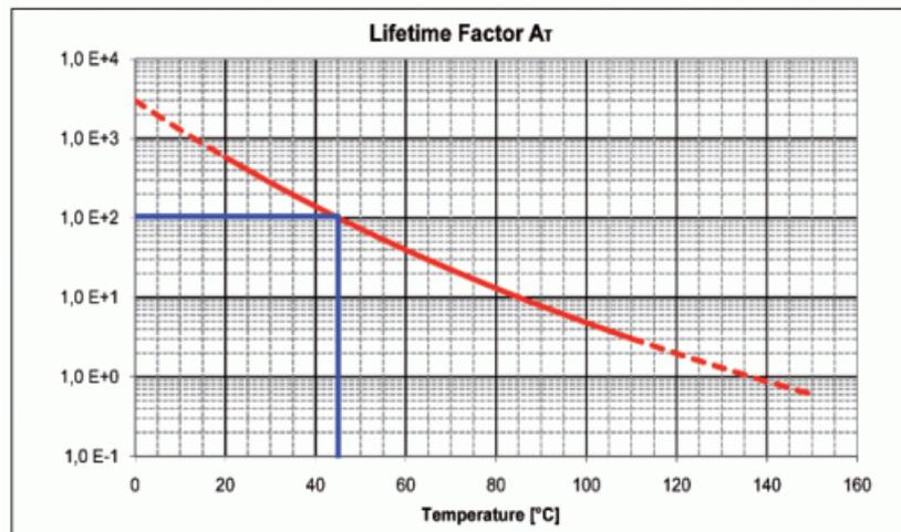
Fig. 9: Interdependency between the mean MTTF of a PICMA® actuator and the ambient temperature
