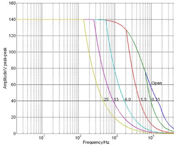
Fig. 6: E-617 open-loop frequency response with various PZT loads. Values shown are capacitance in μF.
