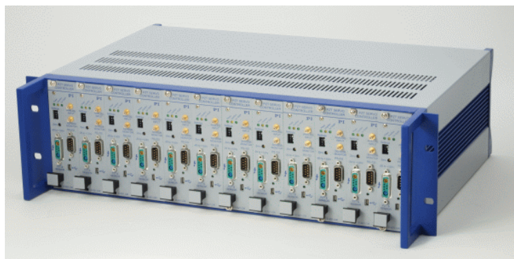
Fig. 1: E-621s installed in compatible PI chassis (E-500.621 in this example) are automatically networked
