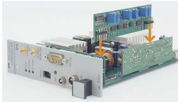
Fig. 9: E-802 servo-control submodule location on E 621. Note and respect component-side orientation.
