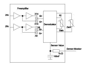
Fig. 16: E-801.20 LVDT submodule sensor readout signal flow. Zero pot is on main module.
