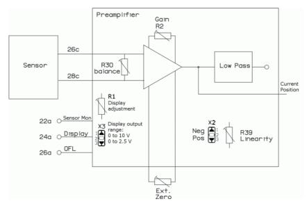
Fig. 8: E801B1008 signal path diagram; Ext. Zero pot is on main module of the controller
