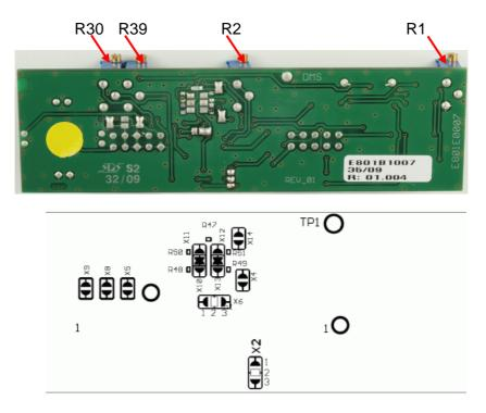
Fig. 7: E801B1007, solder side, with corresponding drawing showing the solder bridges
