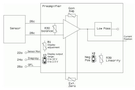
Fig. 13: E801B2008 signal path diagram; Ext. Zero pot is on main module of the controller
