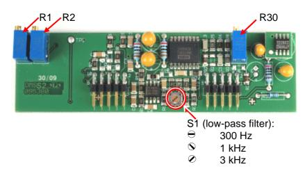
Fig. 3: E-801.10 and .15, component side
