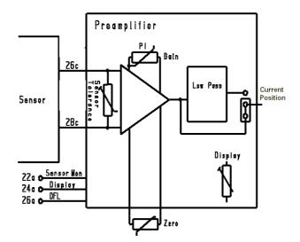
Fig. 2: E-801.10 and .15 signal path diagram; Zero pot is on main module of controller
