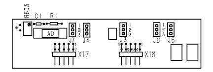
Fig. 17: LVDT conventional (older) version (here E-801.25) with adjustment element location diagram
