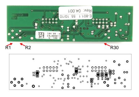
*Fig. 4: E-801.15, solder side, with corresponding drawing showing the solder bridges (with E-801.10, X3 is open and X2 closed, all other elements are identical to E-801.15)*
