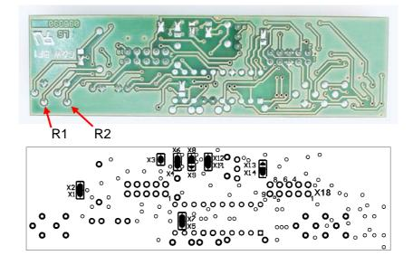
Fig. 19: SMD version, solder side, with corresponding drawing showing the solder bridges that replace the jumpers.
