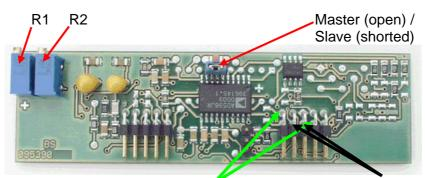
Sensor bridge measuring points, X18 pins 9&4, GND 6&8
