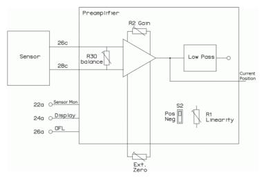
Fig. 11: E-801.30 signal path diagram;Ext. Zero pot is on main module of the controller
