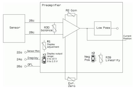
Fig. 5: E801B1007 signal path diagram; Ext. Zero pot is on main module of the controller
