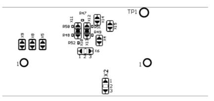
Fig. 15: E801B2008 solder side with solder bridges
