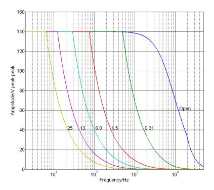
E-625: Operating limits (open loop) with various piezo loads, capacitance values in  $\mu F$
