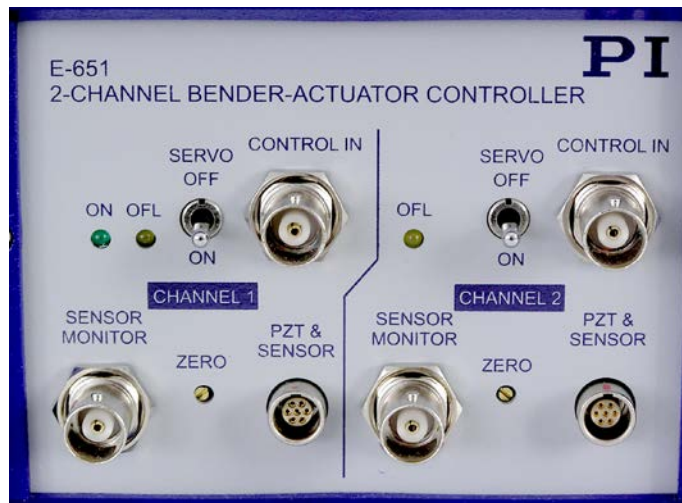
Fig. 2: E-651 front panel; elements for channel 2 are not present on single-channel models
