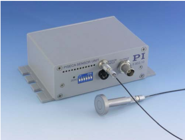
Fig. 1: D-510 Single-Electrode Capacitive Sensor probe with E-852.10 signal conditioner electronics
