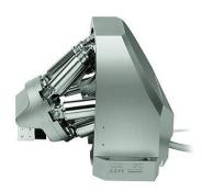
Caption: The double-sided fiber alignment system F-712.HA2 features a H-811 hexapod and a P-616 NanoCube® nanopositioner as basis. The parallel-kinematic design provides high system stiffness. The motorized drives enable longer travel ranges while the NanoCube® nanopositioner ensures fast scanning movements. (Photo PI)
