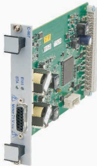
C-867.1xC885 Motion controller module for performance class 3 PLine® piezo motor systems
