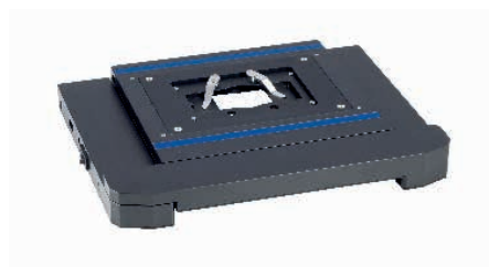
In addition to the fast PLine® ultrasonic motors and high resolution sensor technology, this XY stage also has a fully-fledged controller and can therefore be operated directly with a USB joystick without additional external electronics. It provides an inexpensive solution for automating object motion under benchtop microscopes.
