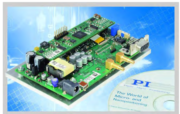
Figure 6. E-709 is available in caseless OEM versions for embedded applications.
